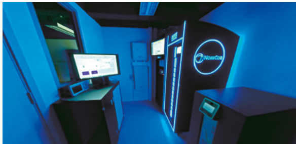
智能電網運行中心配備實時數字仿真系統和功率硬件在環測試平台。 Smart Grid Operation Centre is equipped with Real Time Digital Simulator and Power Hardware-in-the-Loop testing platform.
