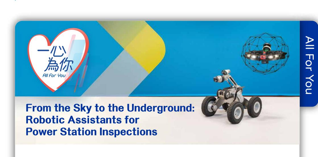
robots for power station inspections. The latest addition to their arsenal are the cage drone and crawler robot, which can inspect above and below ground. The cage drone is small and can fly steadily indoors without GPS.
