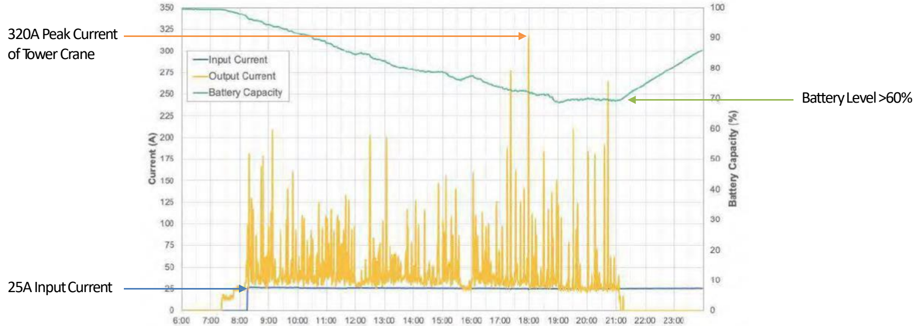
Example: 1-day operation load profile of a BESS supplying two tower cranes
